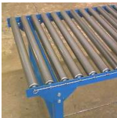
Mild steel frame and rollers
